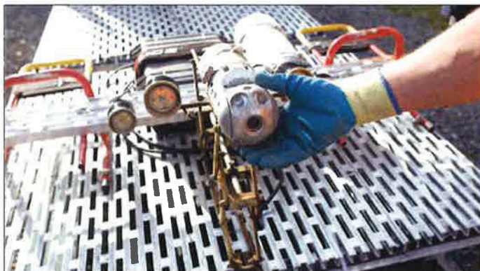
A crew member adjusts a CCTV camera rig. To the left are the LED lights, which are powered by the cylindrical battery pack seen behind the camera.
